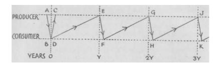
The full lines of the diagram represent the various payments made between producers and consumers in respect of the original construction and subsequent major replacements of any given capital asset, costing £X, and estimated to last Y years.
